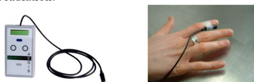
Figure 1. AEGIS ED2 EPD and position of attachment on the index finger
