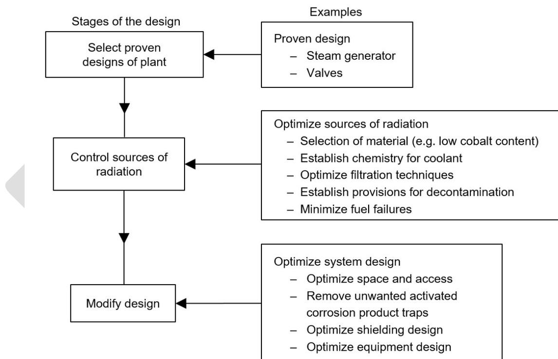
FIG. 2. A simplified strategy for the reduction of exposures in the plant.
