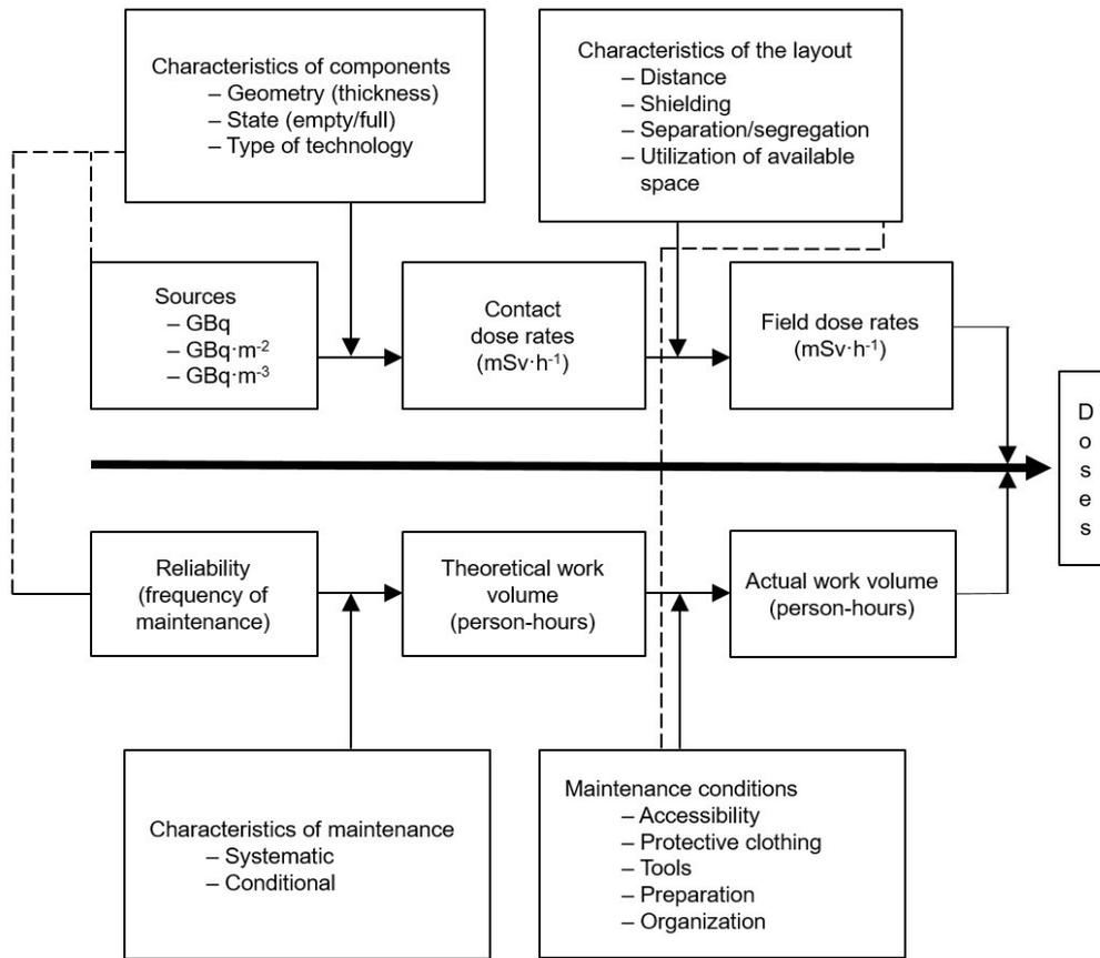
FIG. 3. Schematic flow chart of the origin of doses at a plant (dashed lines indicate the possible impact of certain blocks on others).
