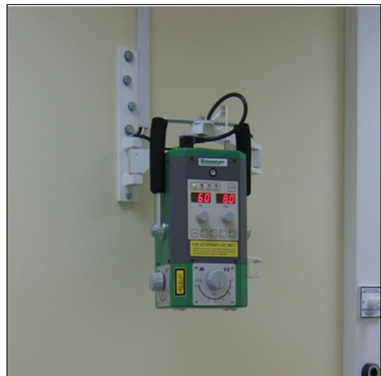
Figure 1 – Adjustable beam collimation and adjustable kV and mAs
